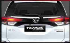
Emergency Stop Signal (ESS) (R All) Otomatis memberi sinyal lampu hazard saat pengereman mendadak.
